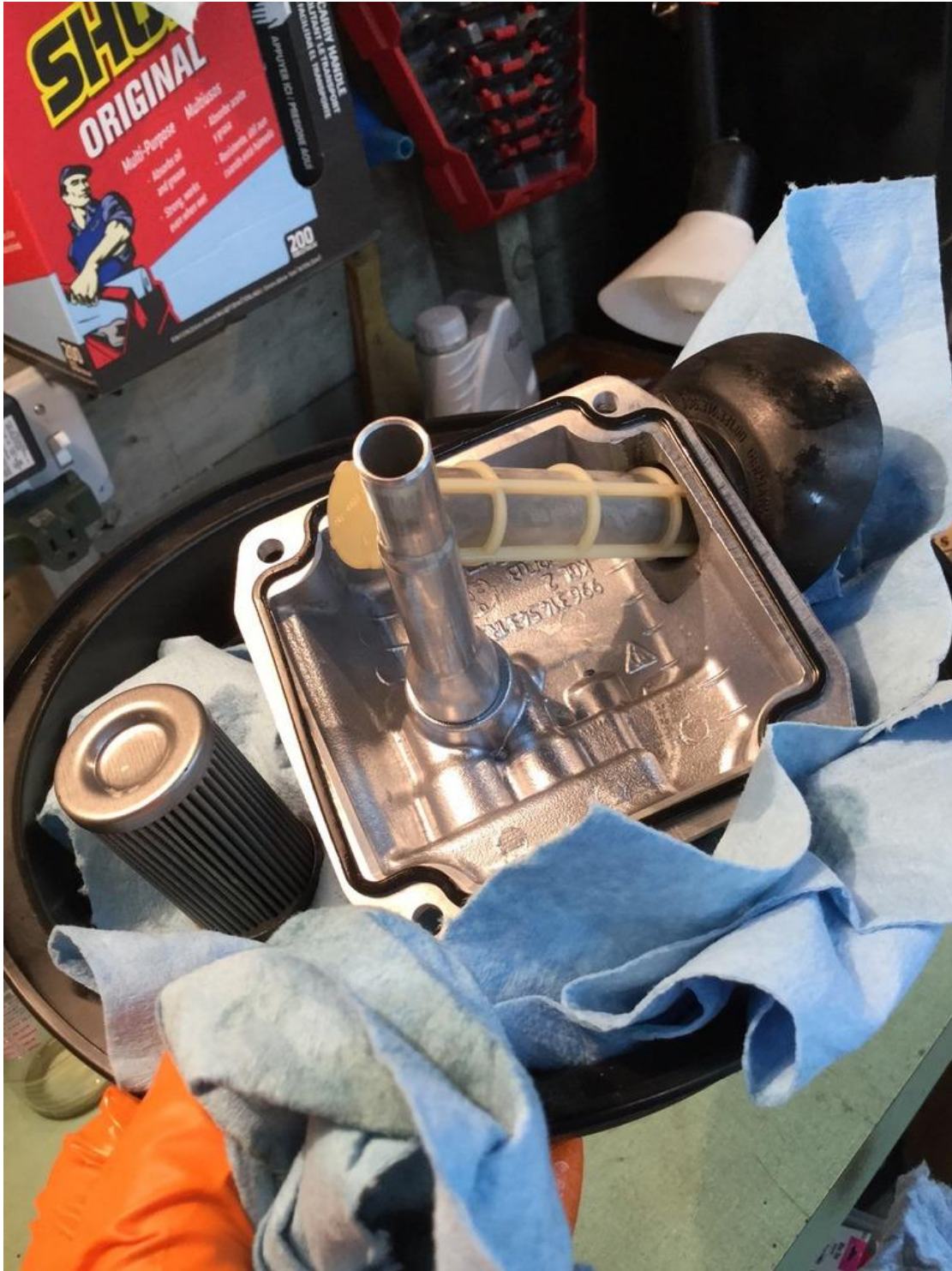
Seven more bolts and the pump is out.
