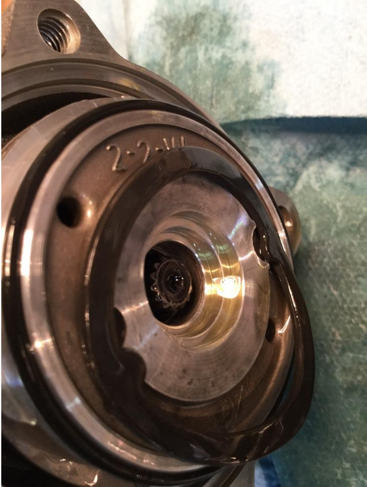
Hard line removed and replaced with beautifully made M12 x 1.0 flare plug. Thank you again, "TheDeckMan" !! :
